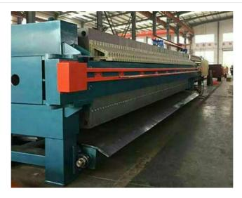
The filter press is affected by acid and alkali corrosion, mechanical wear and the aging of the filter cloth in the process of use, which results in the filter cloth of the filter press has a life limit. Generally, the service life of filter cloth of filter press used in ceramic industry and coal industry is about 3 to 5 months. The service life of filter press cloth used in sludge treatment will be relatively longer.
