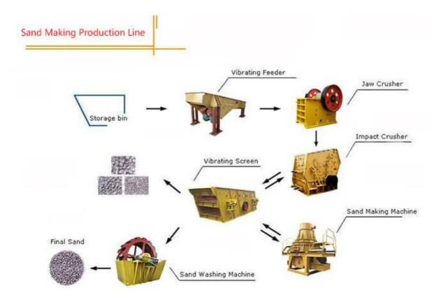
Above is the basic process and the investment budget involved in the setup of a crush sand plant. From the above introduction, it can be found that the medium investment make up a large portion of the crush sand plant.
